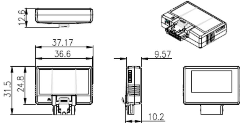
Dimension tolerance:  $\pm 0.2\text{mm}$
